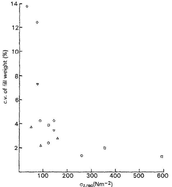
Fig. 3. C.V. of fill weight as a function of  $\sigma_{z, req}$  ('clean' nozzle M). (○) S, (Δ) A, (□) C, (▽) M, (◇) L.
