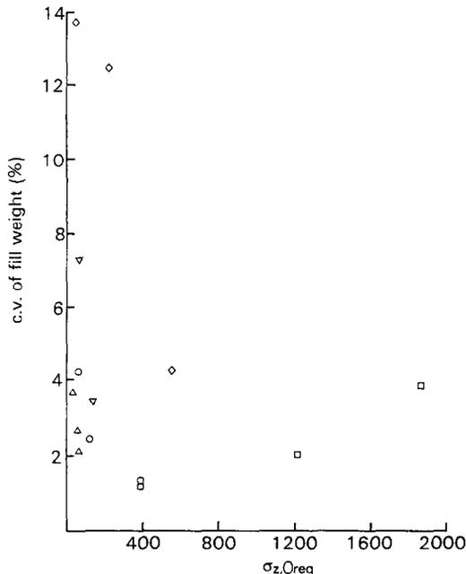
Fig. 4. C.V. of fill weight as a function of  $\sigma_{z,o \text{ req}}$  ('clean' nozzle M). (○) S, (△) A, (□) C, (▽) M, (◇) L.
