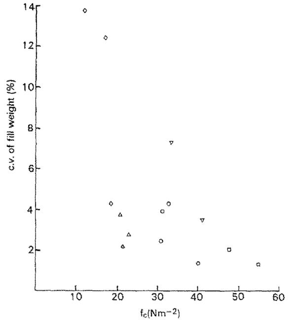
Fig. 2. C.V. of fill weight as a function of  $f_c$  ('clean' nozzle M). (○) S, (Δ) A, (□) C, (▽) M, (◇) L.
